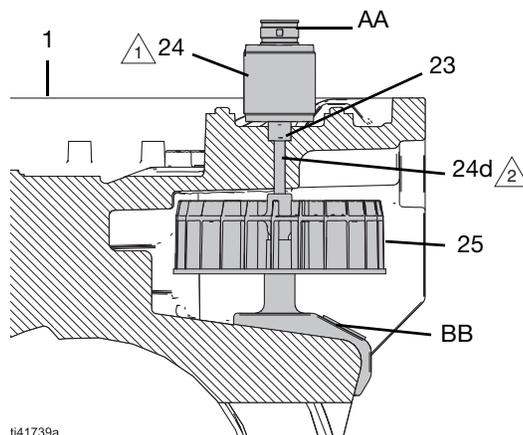
1. Apply thermal paste to the contact surface between the fan motor (24) and stator housing (1).
