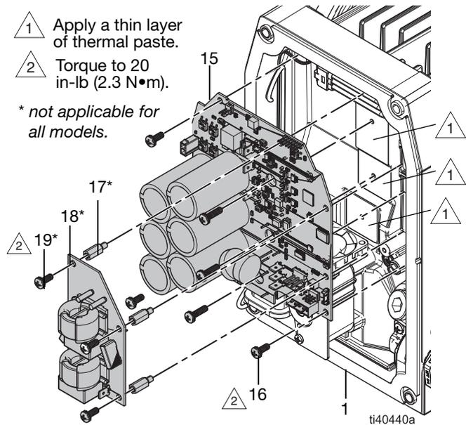
FIG. 10: Control Board and Filter Board
