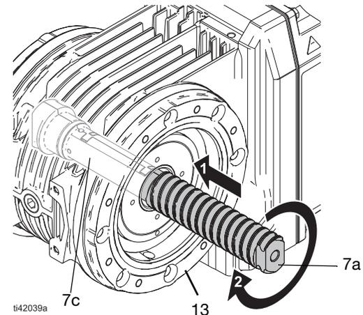
FIG. 18: Remove Rotor Greasing Tool
