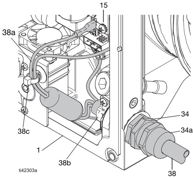
**FIG. 3: Power Cord/Cable (F-2 and F-4 motors)**
