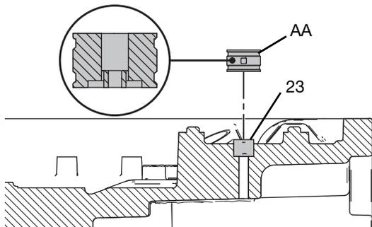
**FIG. 6: Press Bushing on Motor Bearing**
