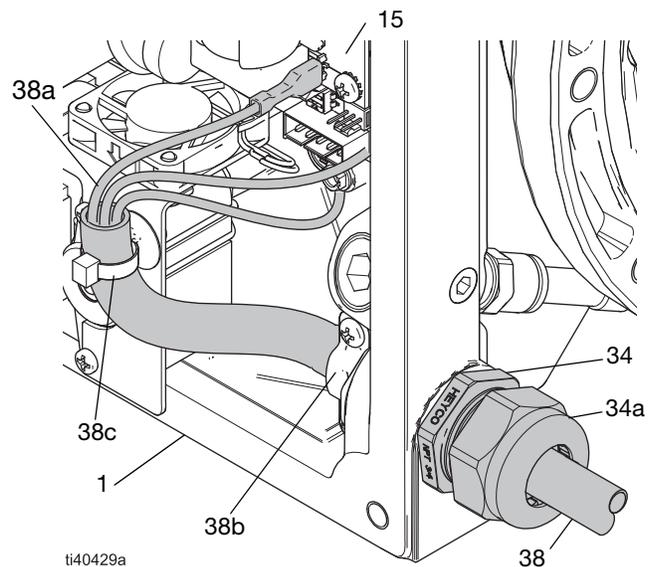
**FIG. 2: Power Cord/Cable (F-1, F-3, F-5, and F-6 motors)**
