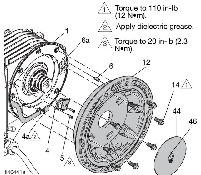
FIG. 11: Motor Sensor
